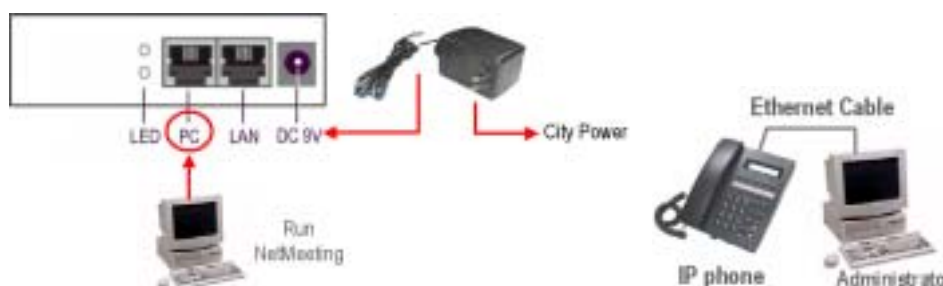
Figure 5.3 To Connect An IP phone to a PC For Call Testing
