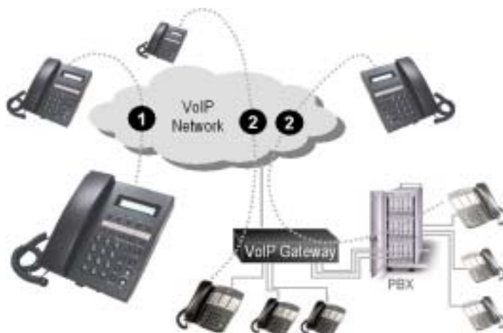
Figure 2.1. The Calling Ways of Phone-to-Phone and Phone-to-Gateway
