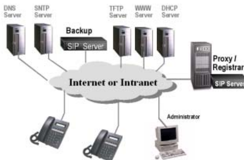
Figure 2.4. The Advanced System Architecture For VoIP Application
