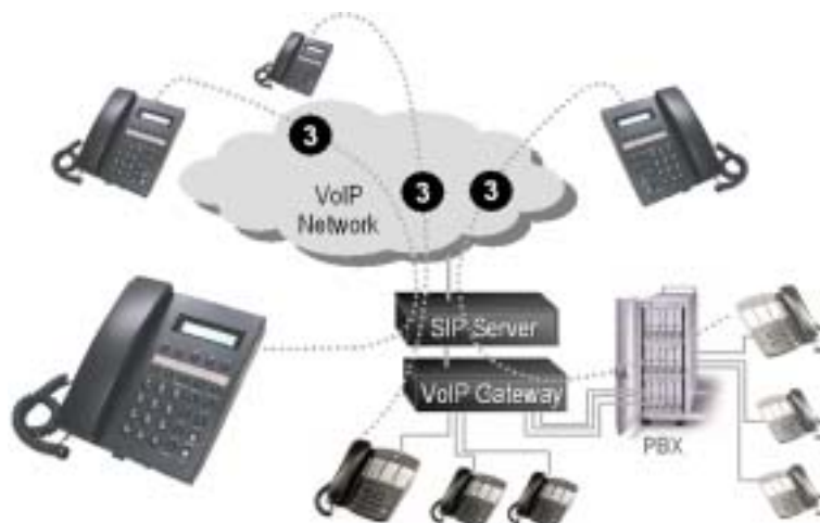
Figure 2.2. The Calling Way of Phone-thru-SIP Server
